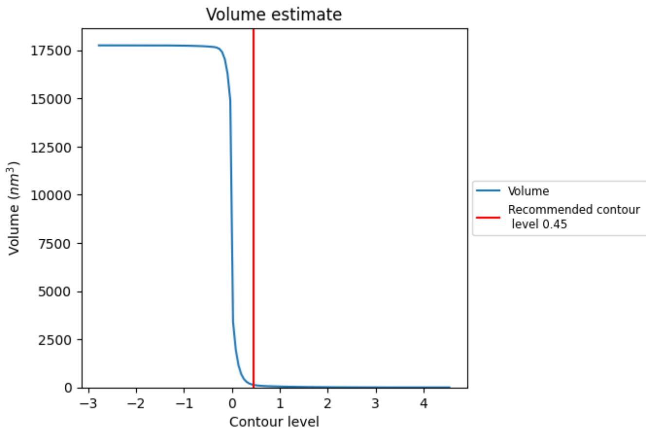
The volume at the recommended contour level is 133 nm<sup>3</sup>; this corresponds to an approximate mass of 120 kDa.
