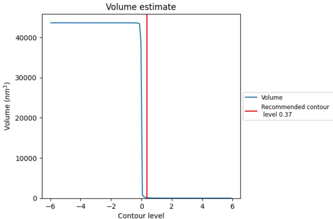
The volume at the recommended contour level is 103 nm<sup>3</sup>; this corresponds to an approximate mass of 93 kDa.
