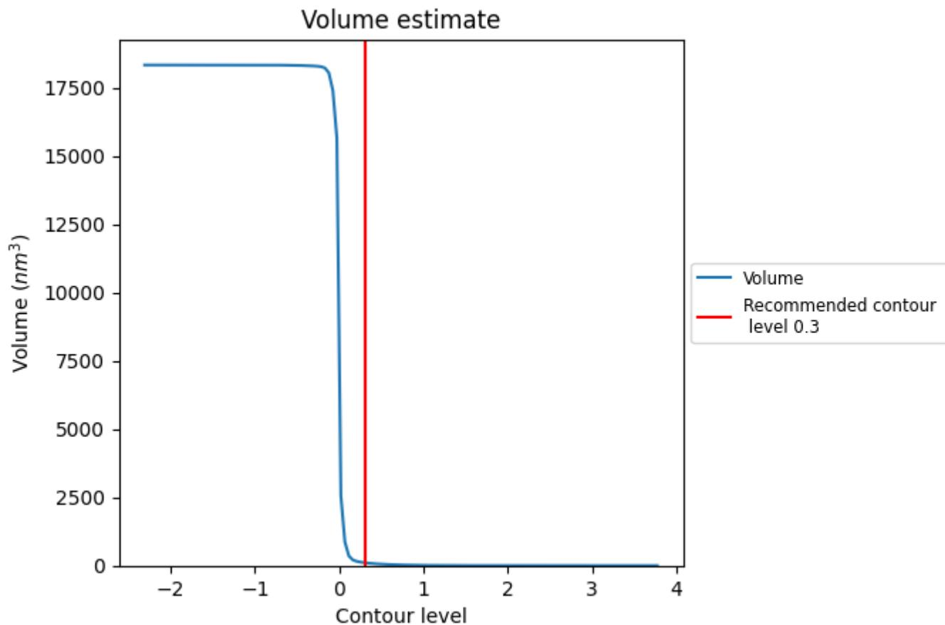
The volume at the recommended contour level is  $106 \text{ nm}^3$ ; this corresponds to an approximate mass of 96 kDa.
