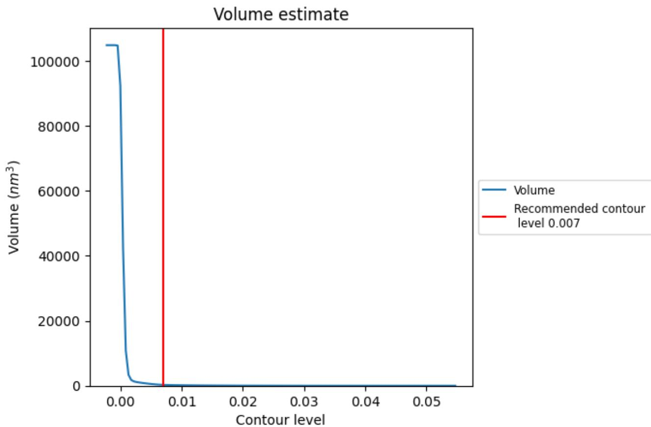
The volume at the recommended contour level is 261 nm<sup>3</sup>; this corresponds to an approximate mass of 236 kDa.
