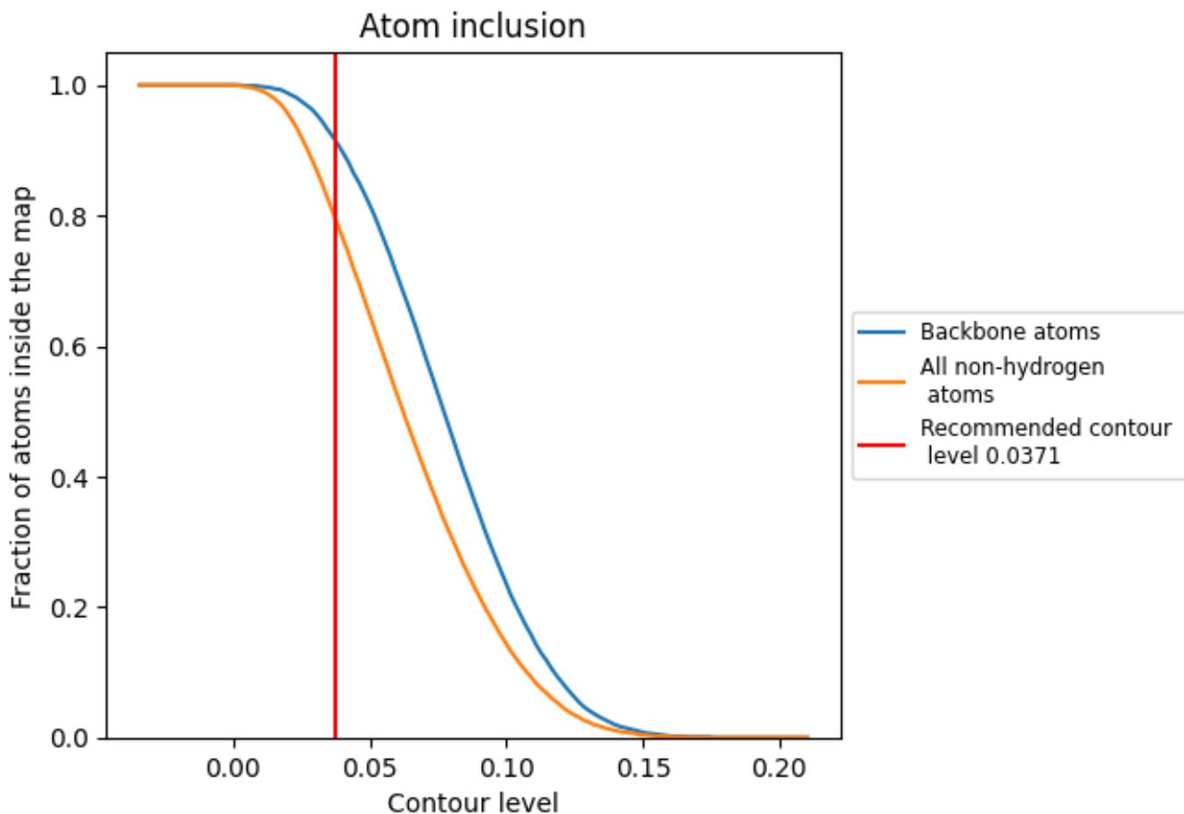
At the recommended contour level, 92% of all backbone atoms, 80% of all non-hydrogen atoms, are inside the map.
