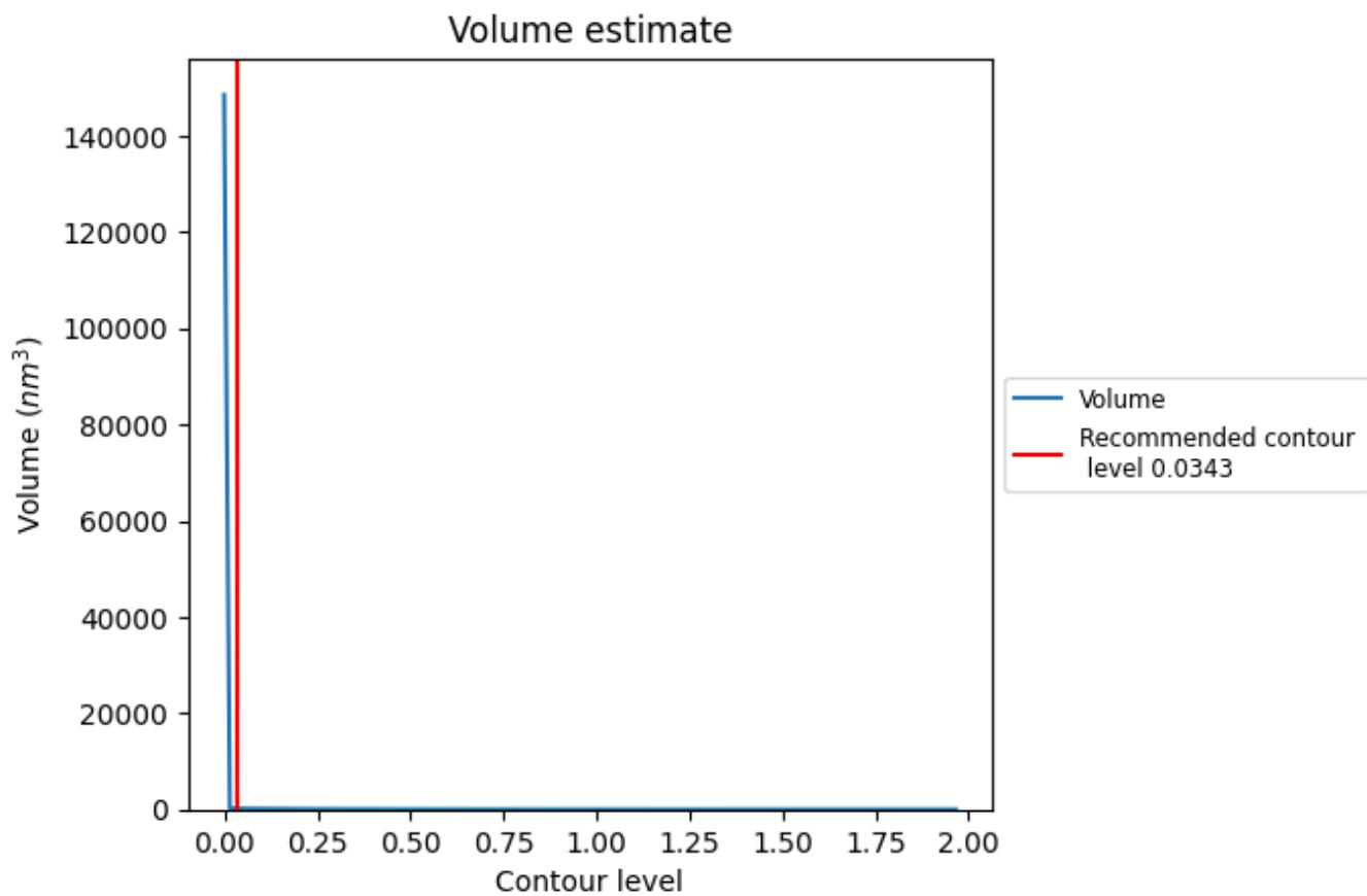
The volume at the recommended contour level is  $188 \text{ nm}^3$ ; this corresponds to an approximate mass of  $170 \text{ kDa}$ .
